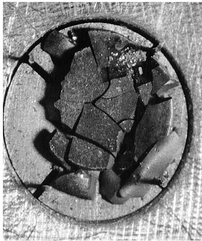
UO 2 discs irradiated to a flat burnup and T_{irr} radial profile. (HBRP project)
