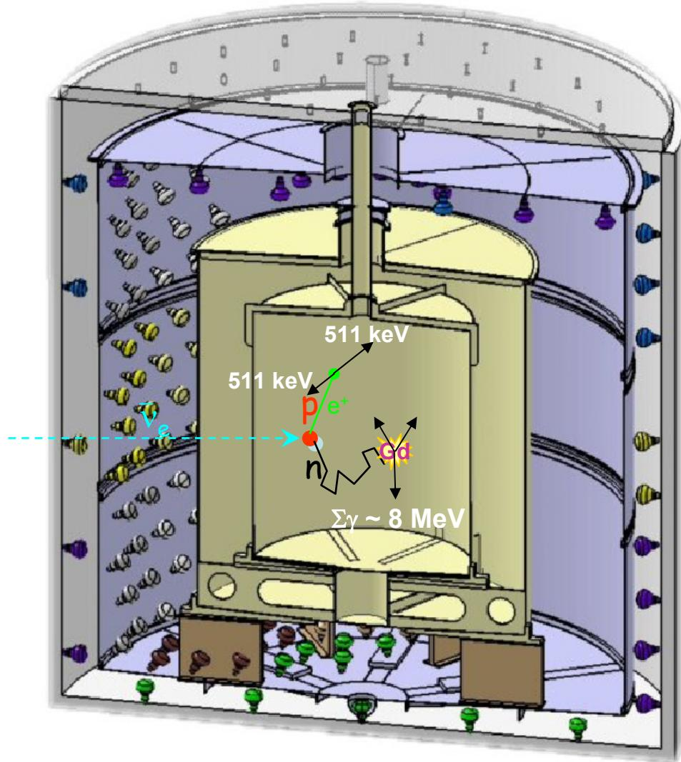
*Signal = Positron signal + Neutron signal after an average of ~30 μsec*
