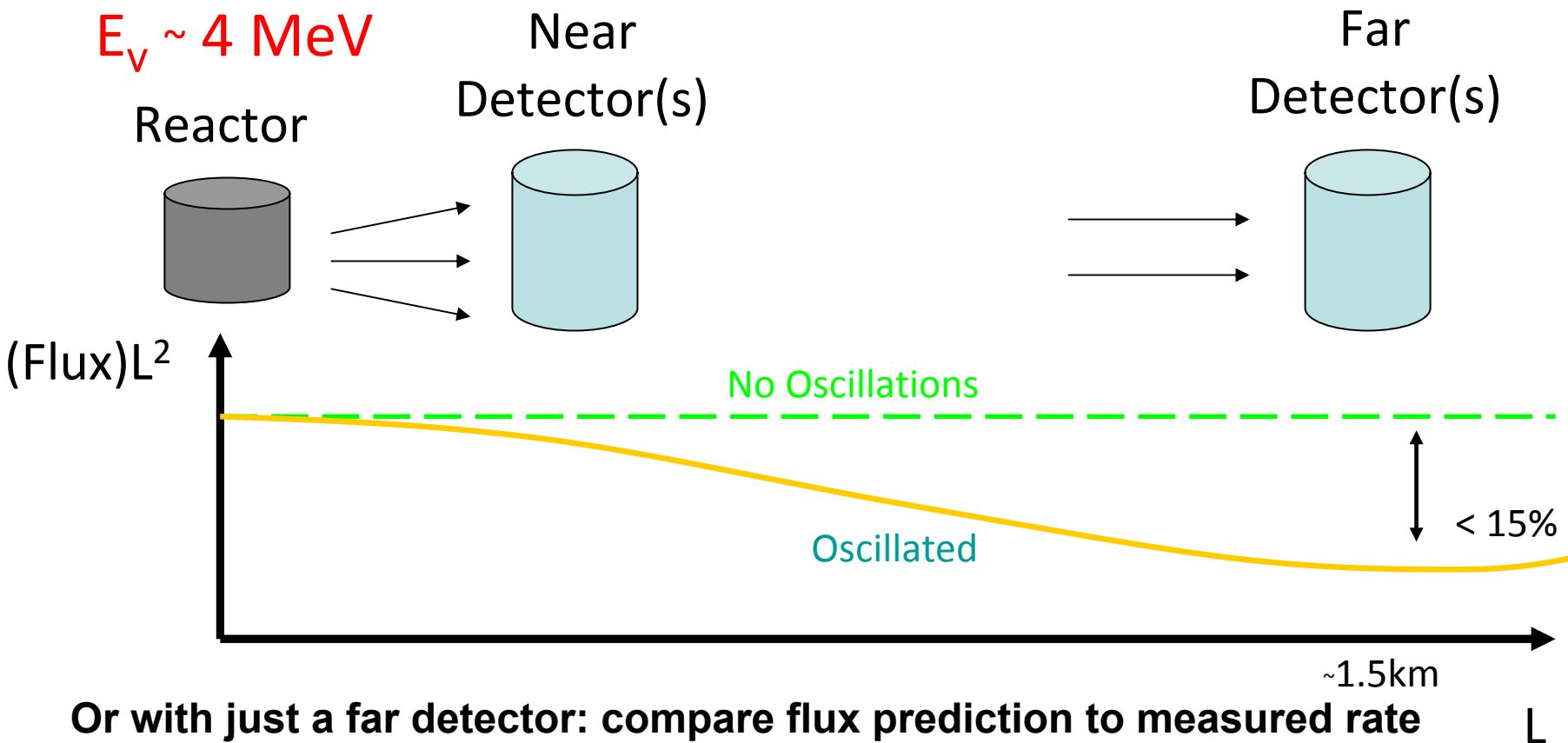
Or with just a far detector: compare flux prediction to measured rate
