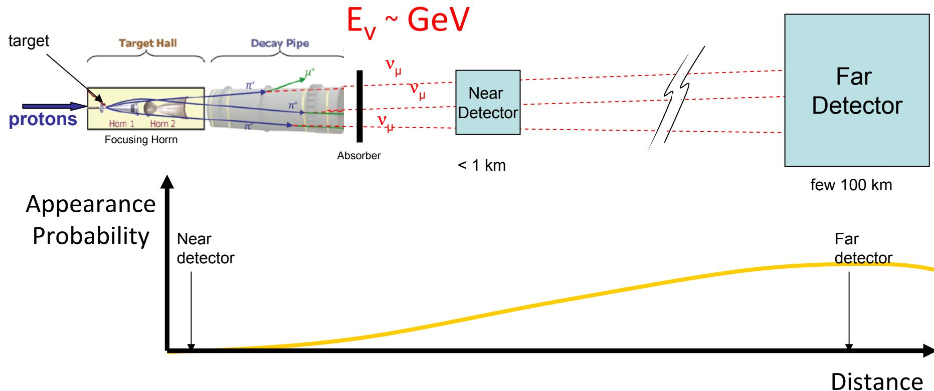
Extrapolate signal/background flux measured in near detector to far detector
