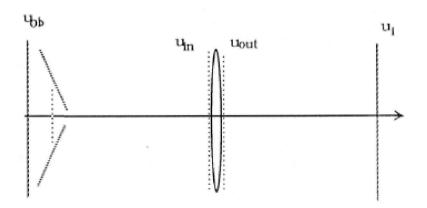
$u_{ob}$  field, complex amplitude, from object  $u_{in}$  field on input plane of the lens (entrance pupil),  $u_{out}$  field after the lens (exit pupil)  $u_{i}$  field on image plane (e.g. as defined by geom. optics)
