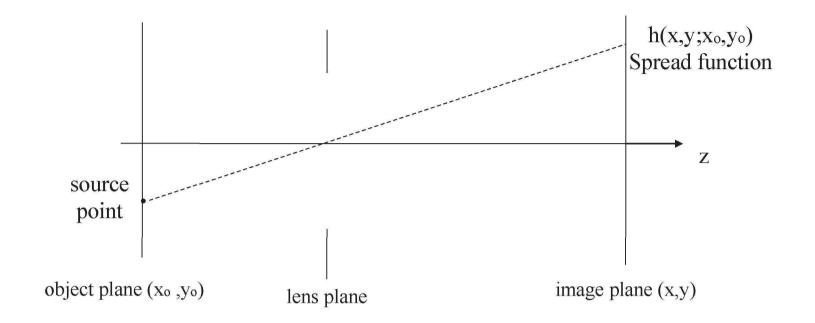
Let us assume to have an extended source. Let  $u_{ob}(x_0,y_0)$  be the complex amplitude distribution density (surface density). Each element  $dx_0dy_0$  gives a contribution to the field at x,y, given by
