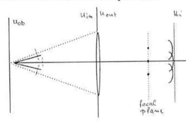
Let us consider decomposition of diffracted field in plane waves (Fourier). Each plane wave is focused by the lens at focal plane.
