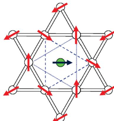
**DM induces canting of Mn3 spins, resulting in polarization due to exchange striction**
