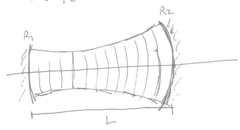
Since the wavefronts of Hermite-Gaussian are the same as for Gaussians, spherical pairs of mirrors that support Gaussian beams also support Hermite-Gaussian beams. For any m,n, support Hermite-Gaussian beams. For any m,n, therelation between Zolza and L,R, LRz are the therelation between Zolza and L,R, LRz are the same as for Gaussian beams. However, the same as for Gaussian beams. However, the allowed frequencies change slightly:
