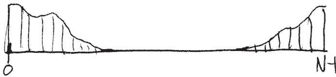
To reconstruct  $\tilde{f}(v)$  we must cut the second half and place it before the first. we also need to multiply by  $\sqrt{N}\Delta x$ .
