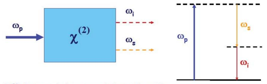
≈10<sup>10</sup> photon pairs/sec generated over the entire emission cone by 100 mW UV in few mm of NL crystal
