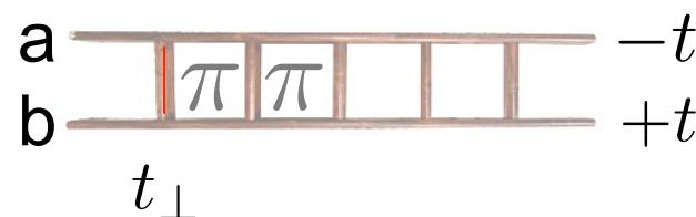
$$H = -t \sum_x (a_x^\dagger a_{x+1} + a_{x+1}^\dagger a_x) + t \sum_x (b_x^\dagger b_{x+1} + b_{x+1}^\dagger b_x) - t_{\perp} \sum_x (a_x^\dagger b_x + b_x^\dagger a_x) + \frac{U}{2} \sum_x (n_{a,x}^2 + n_{b,x}^2)$$
