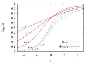
Spin 0 condensate fraction  $n_0/(n/2)$  as a function of the adimensional interaction strength  $y=1/(k_Fa_s)$  for three values of v and two values of  $\theta$ :  $\theta=0$  means  $v_R=v$  and  $v_D=0$  (red solid curves), while  $\theta=\pi/4$  means  $v_R=v_D=v/\sqrt{2}$  (blue dotted curves). v is in units of the Fermi velocity  $v_F=(3\pi^2n)^{1/3}$ .
