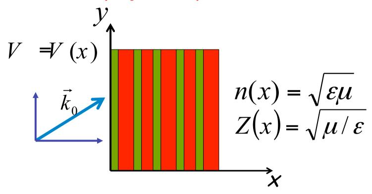
Quasiparticles with the energy W in a graphene super-latice created by a electrostatic potential V(x)
