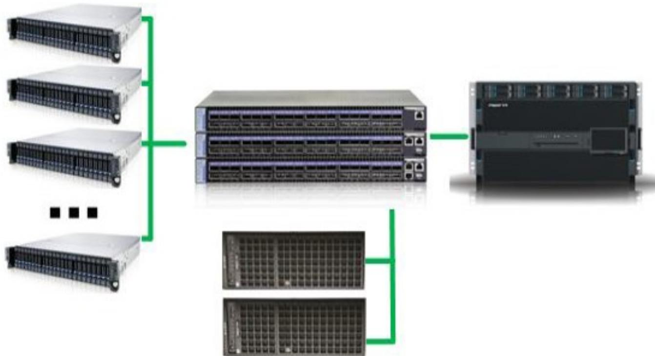
World-class InfiniBand switches provide full wire-speed 40Gb network interconnection for all compute nodes.
