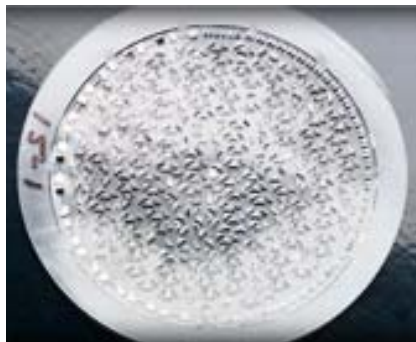
Electroplated LIGA mold
