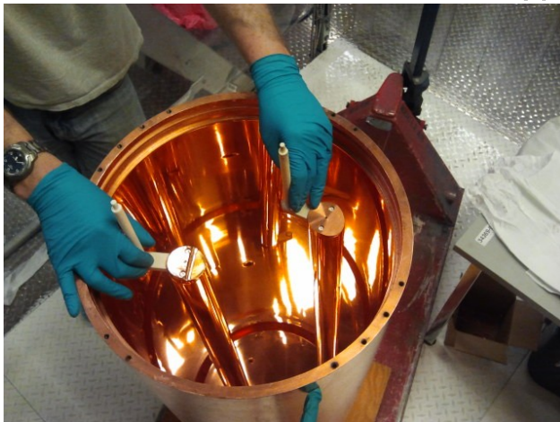
Cavity with lid off, showing tuning rods
