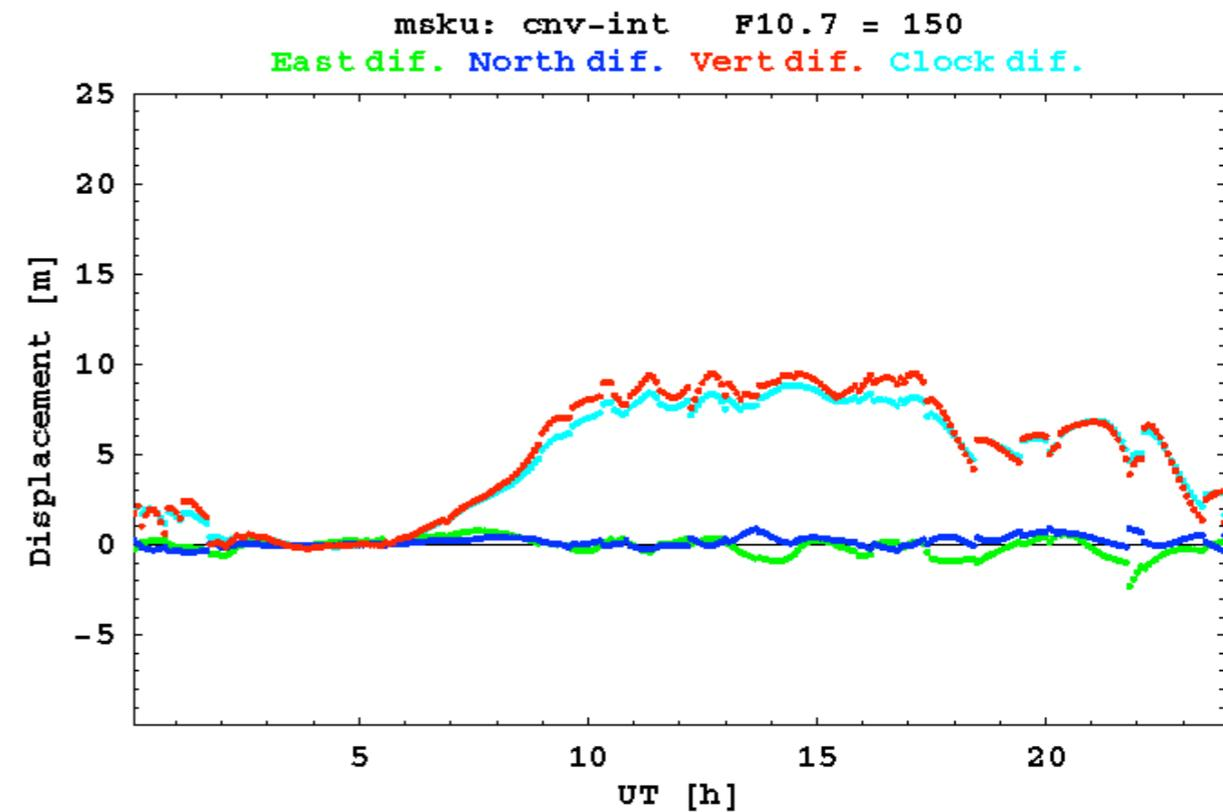
Mapping function errors effects at **position domain** for different levels of solar activity in a low latitude station: Franceville ( $-2^\circ$  N,  $14^\circ$  E).
