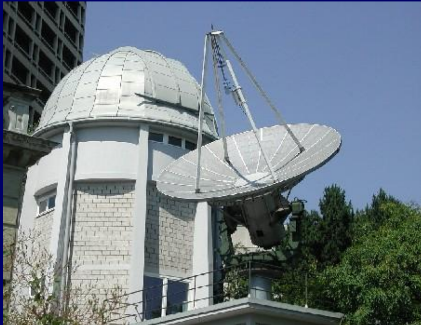
Antenna at sun tower of Zurich observatory pointing to the sun
