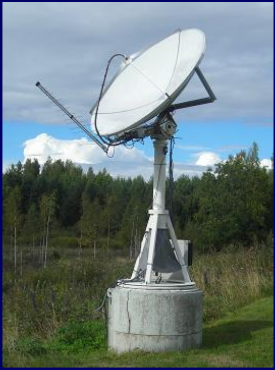
DVB-T log-per attached to a 37 GHz microwave-dish
