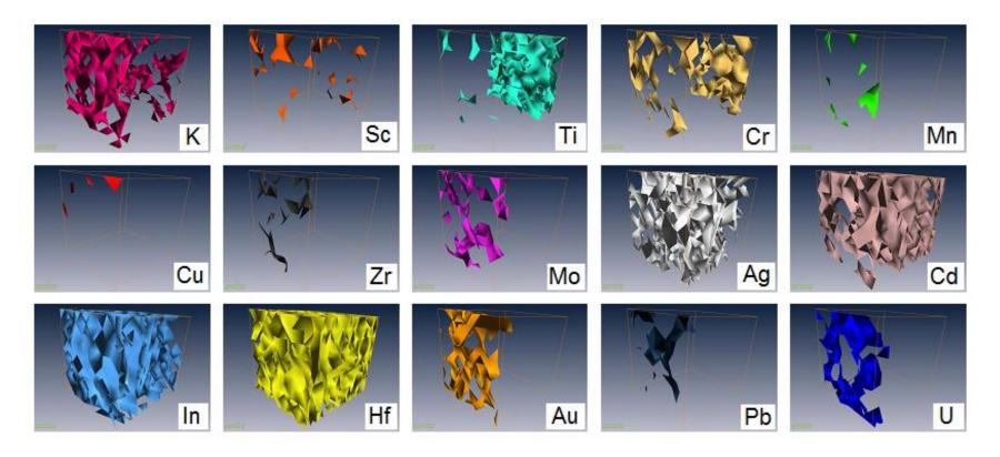
HASYLAB, DESY, DORIS III, beamline L NIST SRM 611 glass standard. Scanned volume: 135  $\mu$ m / 135  $\mu$ m / 150  $\mu$ m Incident X-ray beam: 6.7  $\mu$ m, 21 keV.
