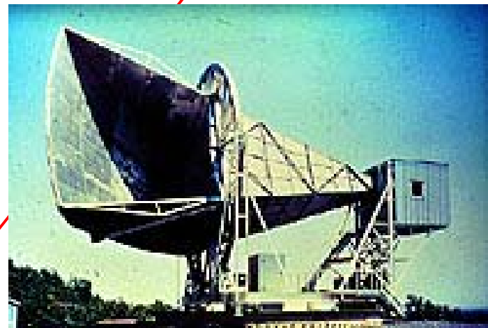
Fig. 12. — Upper panel: scheme of the horn-antenna. It is a part of a large paraboloid: lateral shields prevent spurious radiation entering in the system outside the nominal beam width. Isotropic level -43 dB. Lower panel: angular response of the antenna, as measured by means of a transmitter located in front of the antenna at different angles. The spillover lobe is studied in detail in the lowest part of the graph. Earth's radiation entering via the spillover lobe determines the antenna temperature noise. — Measured data, ● computed data. (Adapted by Crawford et al. [34].)
