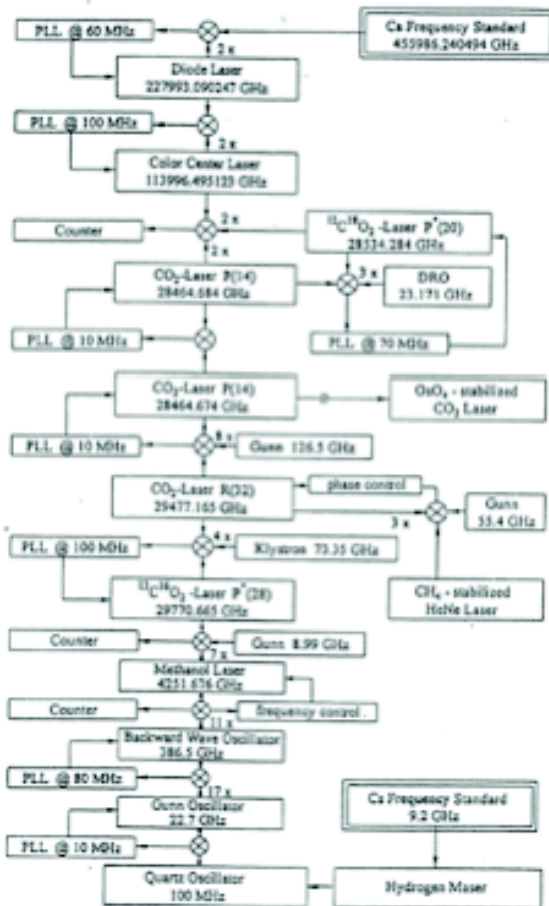
FIG. 1. PTB's frequency chain to the Ca intercombination line (PLL = phase locked loop, details are given in the text).
