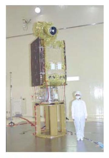
Fig. 5. LUCE LCT on top of the OICETS spacecraft.
