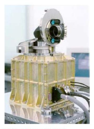
Figure 1: TESAT LCT for 45,000 km LEO-GEO links at 1.8 Gbps
