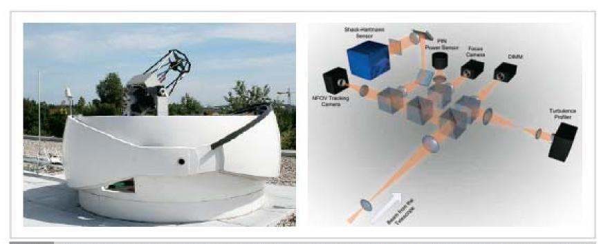
Fig. 2 Image of receiver telescope in June 2009, hosted by an astronomical clamshell dome (left) and Instrument setup in the 2009 campaign (right). The beam is guided to the tracking camera, receiver frontend and measurement instruments [5]
