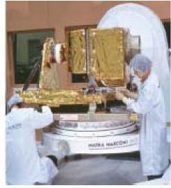
Fig. 4. ARTEMIS (left) and SPOT-4 (right) LCTs during assembly at Astrium SAS (former Matra Marconi Space) France.
