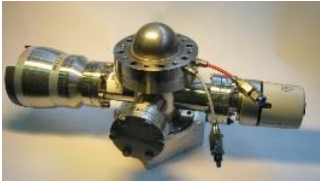
KMC-2 at BESSY-II: custom-build Beryllium dome furnace with double sided borolectric® heater reaches temperatures up to 1000 °C in vacuum ( < 10^{-9} mbar)
