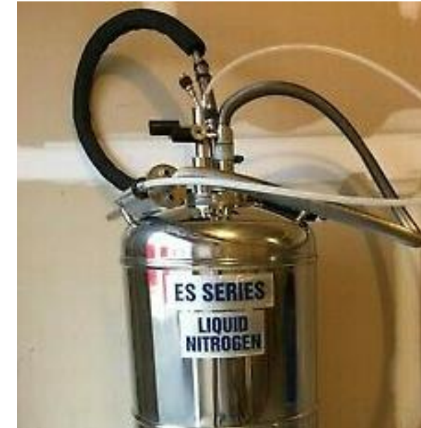
Cryojet for cooling sample (~95 K)
