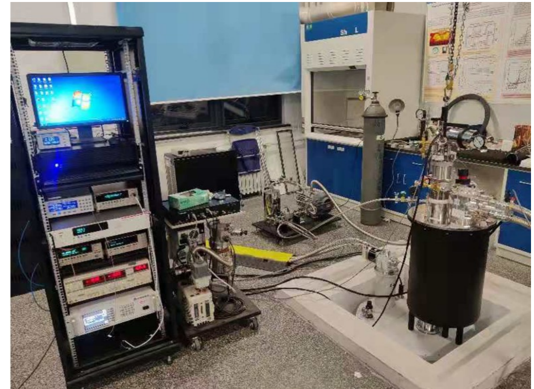
Integrated facility with HP/LT(0.3K)/MF(14T)
