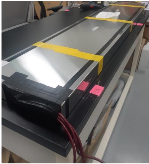
Two panels are installed in a box made of steel frame and aluminum sheets
