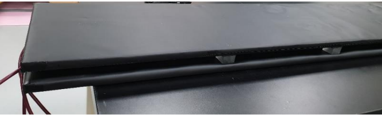
Two complete panels are mounted together with supporter in between (acrery blocks)
