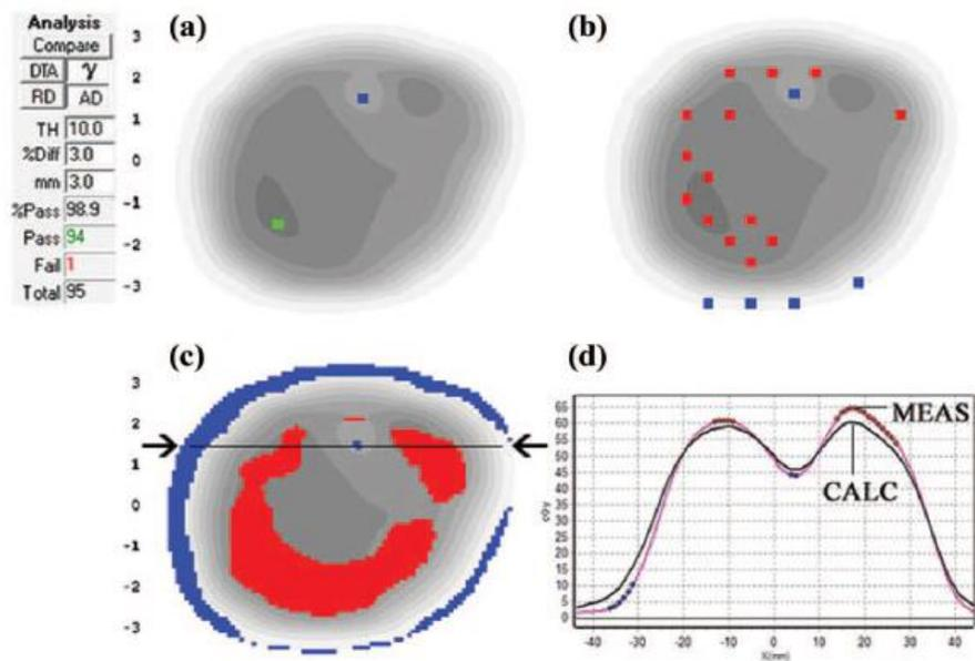
FIG. 3. (a) 3%G/3 mm gamma failing points and (b) 2%L/2 mm gamma failing points based on a diode array at 5 cm depth, 100 cm SDD. In both (a) and (b), the visible dots represent failing points. (c) 2%L/2 mm gamma failing points for EPIDose analysis at same virtual depth and (d) dose profile through the horizontal line indicated by the arrows in panel (c), with the black line extracted from the TPS dose grid and the line with dots highlighted from the measurement.
