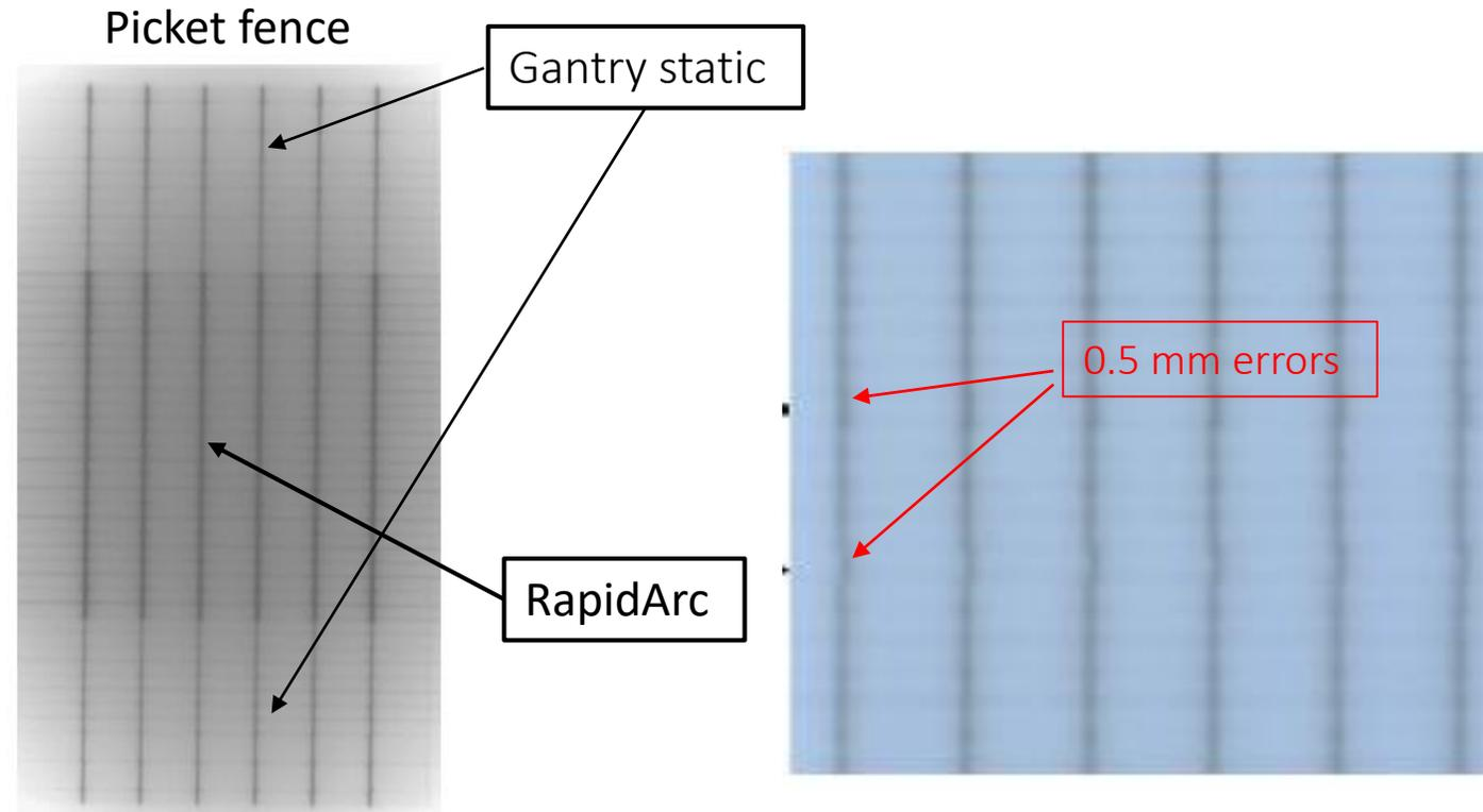
Fig. 3. Image of a film that was exposed twice to the 1-mm-wide picket fence pattern, once at stationary gantry angle and a second time in RapidArc mode.
