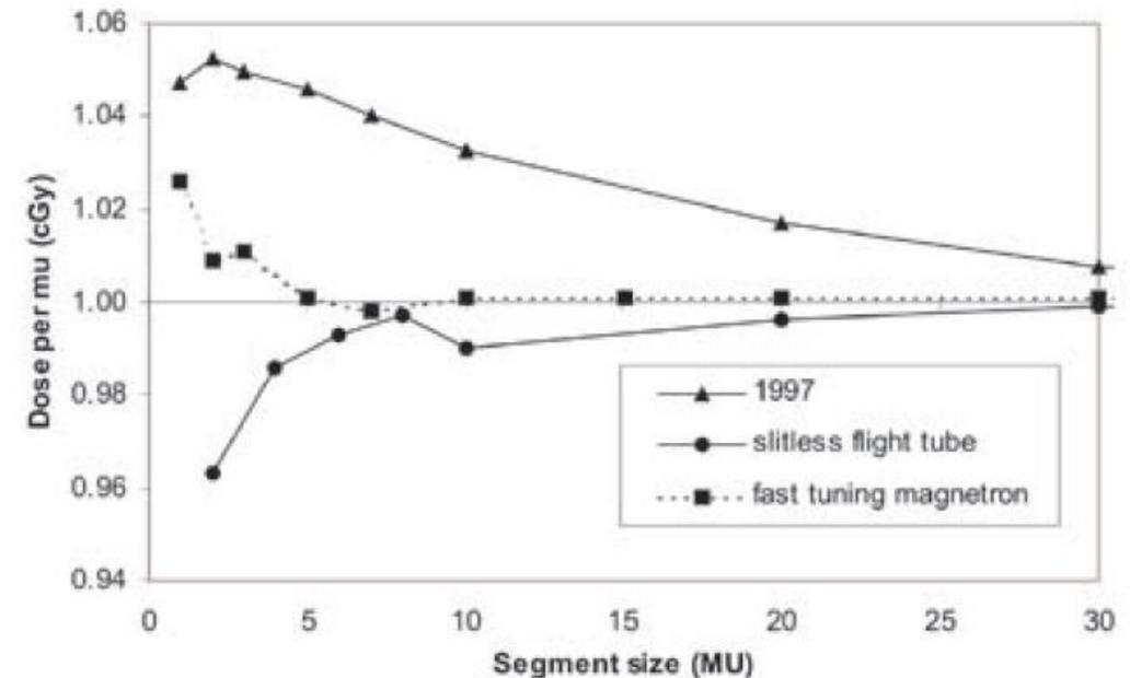
**Figure 4.6** Beam calibration for a limited number of monitor units depending on the type of magnetron and steering technique for Elekta accelerators. In 1997 the feedback technique with slits was used. An improvement of this technique was the slitless flight tube, which was followed by a new design magnetron with faster tuning (Courtesy Geoff Budgell, Christie Hospital, Manchester, UK).
