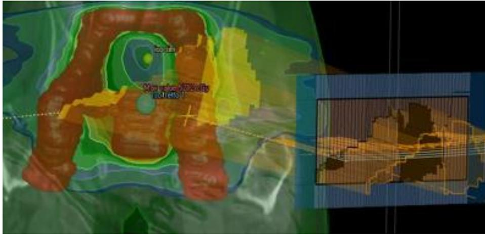
Physical and dosimetric aspects of a multileaf collimation system used in the dynamic mode for implementing intensity modulated radiotherapy
