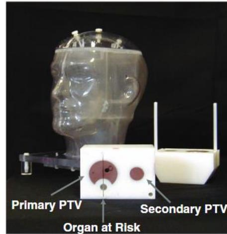
FIG. 1. RPC H&N phantom for IMRT credentialing.
