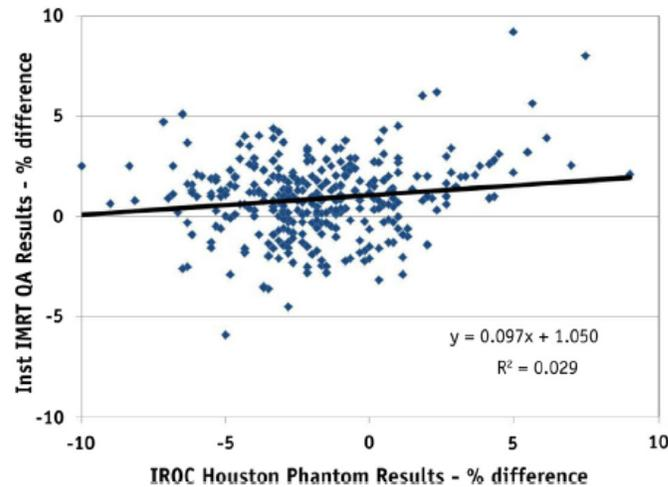
**Fig. 3.** Percent differences between dose measurements and treatment planning system calculations for institutional IMRT QA compared with the TLD in the IROC Houston phantom. The linear trend line should ideally have a slope of 1 but instead is nearly flat. IMRT QA = intensity modulated radiation therapy quality assurance; IROC = Imaging and Radiation Oncology Core; TLD = thermoluminescent dosimeters.
