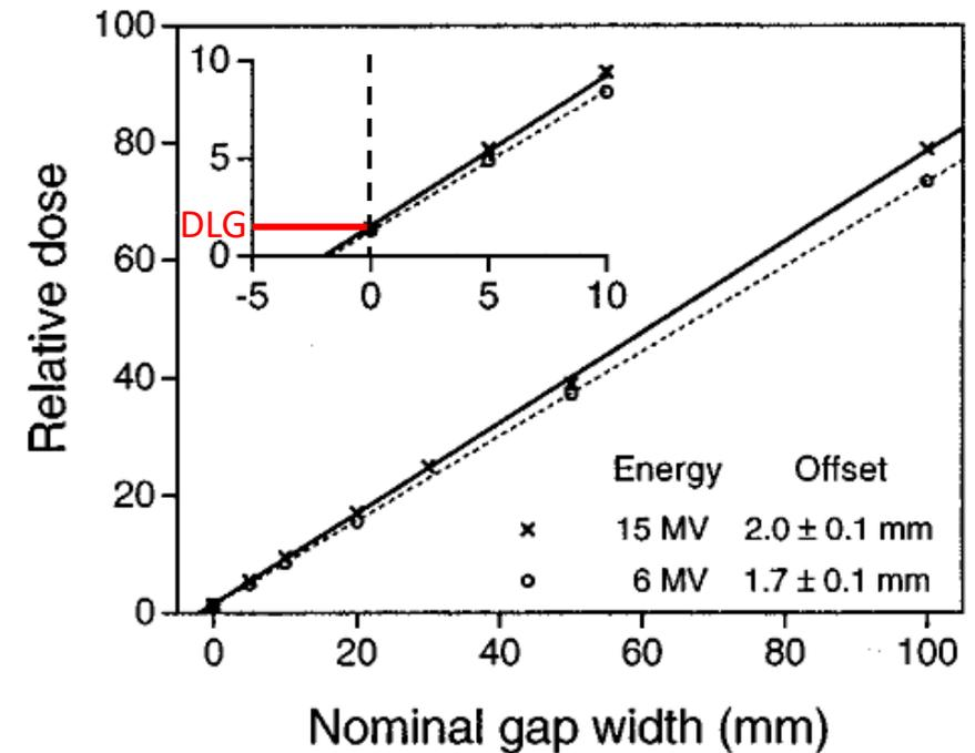
FIG. 7. Integrated dose vs MLC gap width measured in phantom with radiographic film for 6 and 15 MV x rays. The lines are linear fits to the data using least-squares regression. Extrapolation to zero integral dose determines the effective gap offset. The uncertainties are the standard errors of the data.
