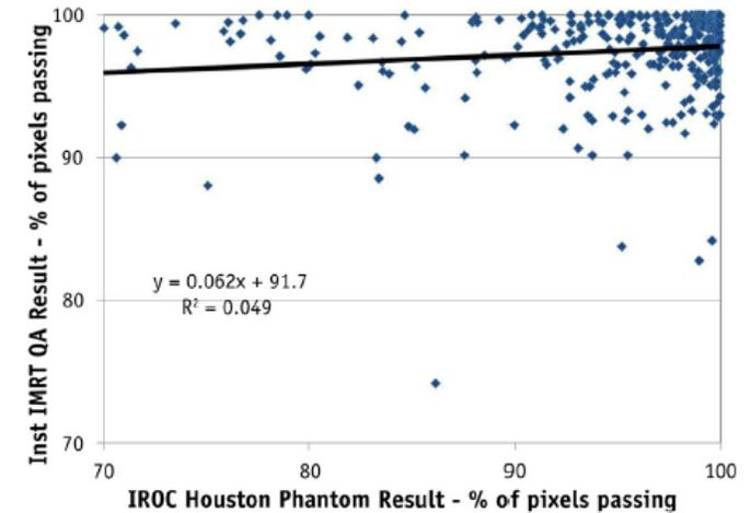
**Fig. 4.** Percent of pixels passing gamma for institutional IMRT QA compared with the IROC Houston phantom films. The linear trend line should ideally have a slope of 1, but instead is nearly flat. IMRT QA = intensity modulated radiation therapy quality assurance; IROC = Imaging and Radiation Oncology Core.
