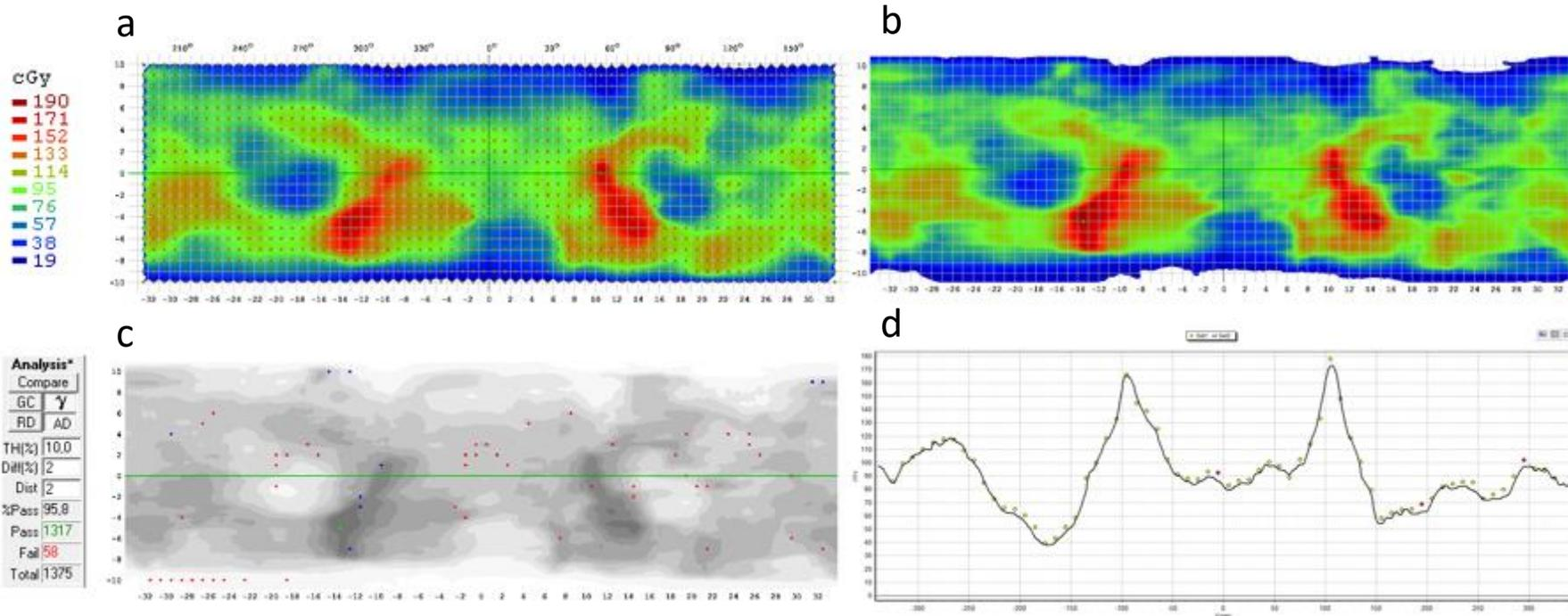
2%/2mm gamma failing points based on the ArcCheck diode Array. The agreement between calculated (b) and measured dose (a) is good (PR=95.8). A slightly systematic underestimation of the delivered dose is visible in c) and d)
