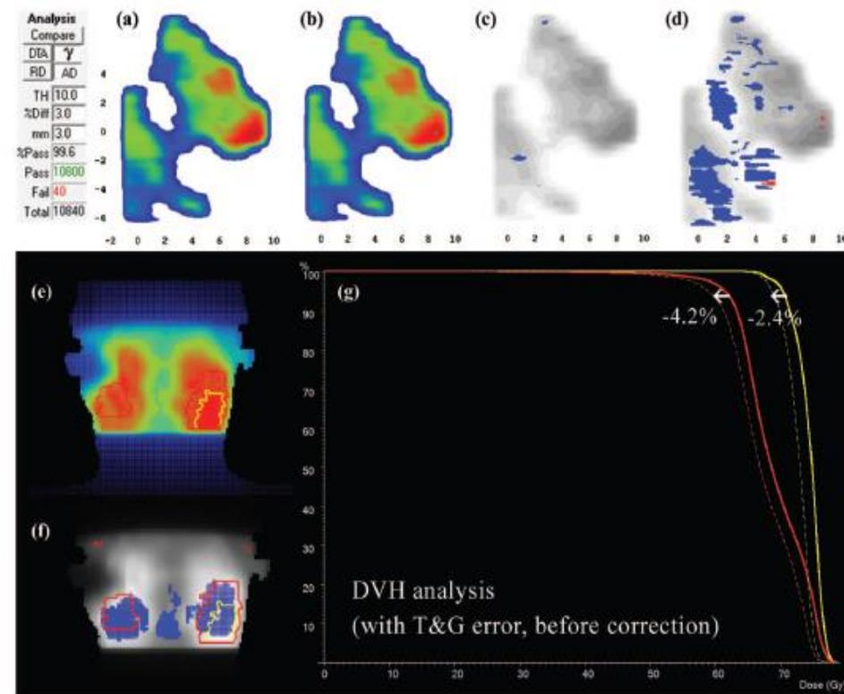
FIG. 2. Absolute dose planes at 5 cm depth, 100 cm SDD for (a) measured and (b) calculated dose. (c) 3%G/3 mm gamma with failing points shown as the shaded region over the calculated plane in grayscale. (d) 2%L/2 mm gamma failing points showing a clear pattern of meas < calc, i.e., shaded regions showing gamma failing points. (e) Patient coronal TPS plane, (f) 3DVH-estimated dose differences (3DVH-TPS), and (g) estimated DVH errors showing lower MGDR target dose compared to planned.
