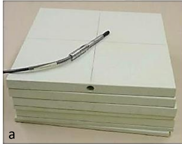
Water equivalent phantom with (a) Farmer-type ion chamber and (b) parallel-plate chamber
