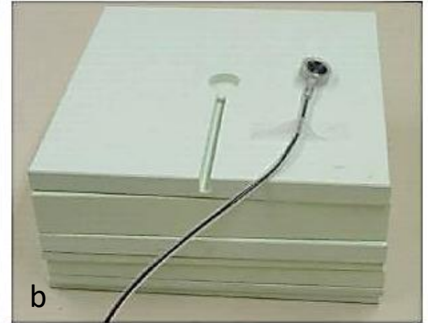
Water equivalent phantom with (a) Farmer-type ion chamber and (b) parallel-plate chamber
