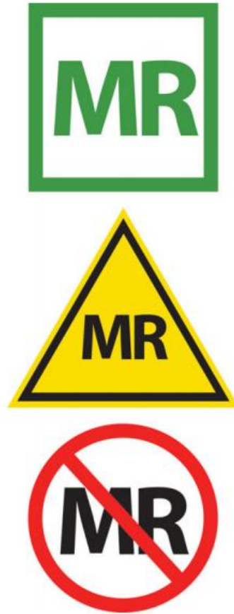
Figure 2. U.S. Food and Drug Administration labeling criteria (developed by ASTM [American Society for Testing and Materials] International) for portable objects taken into Zone IV. Square green “MR safe” label is for wholly nonmetallic objects, triangular yellow label is for objects with “MR conditional” rating, and round red label is for “MR unsafe” objects.
