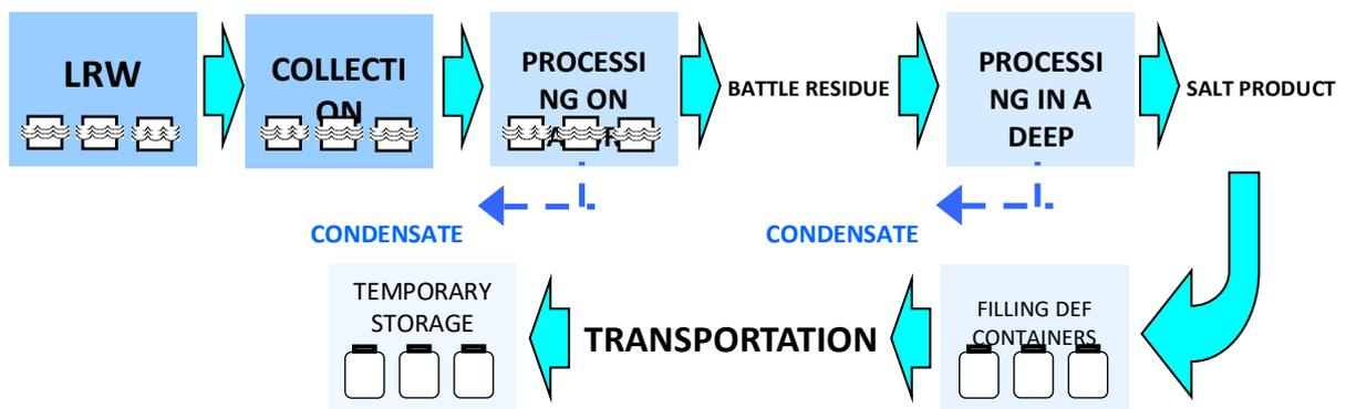
Liquid radioactive waste is processed on water purification system evaporators. To reduce the volume of LRW at the deep evaporation facility (DEF), the distillation residue is processed to a salt concentrate, which is poured into metal barrels in a hot molten state, turning into a monolith after cooling.
