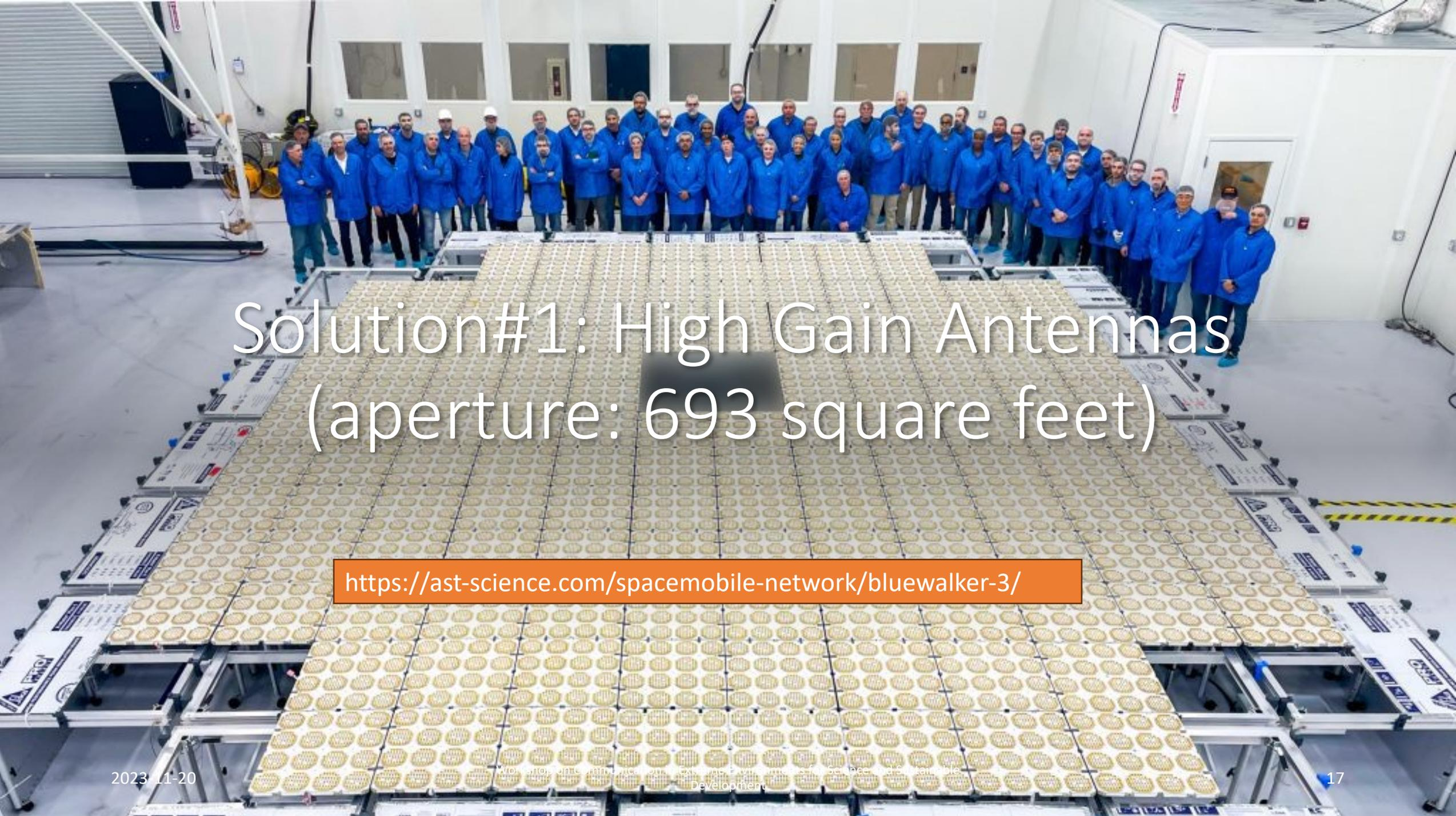
A large group of approximately 50 people, mostly men, are standing in a cleanroom behind a massive array of high-gain antennas. The antennas are arranged in a long, rectangular grid, with each element being a small, circular, gold-colored structure. The people are wearing blue lab coats, and the cleanroom has white walls and a grey floor. The text "Solution#1: High Gain Antennas (aperture: 693 square feet)" is overlaid in white on the image.
