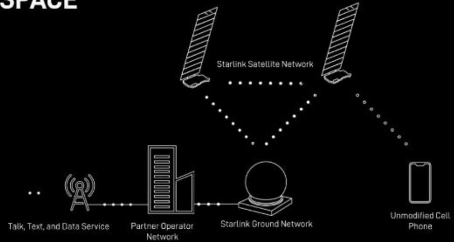
Starlink satellites with Direct to Cell capability have an advanced eNodeB modem onboard that acts as a cellphone tower in space, allowing network integration similar to a standard roaming partner.
