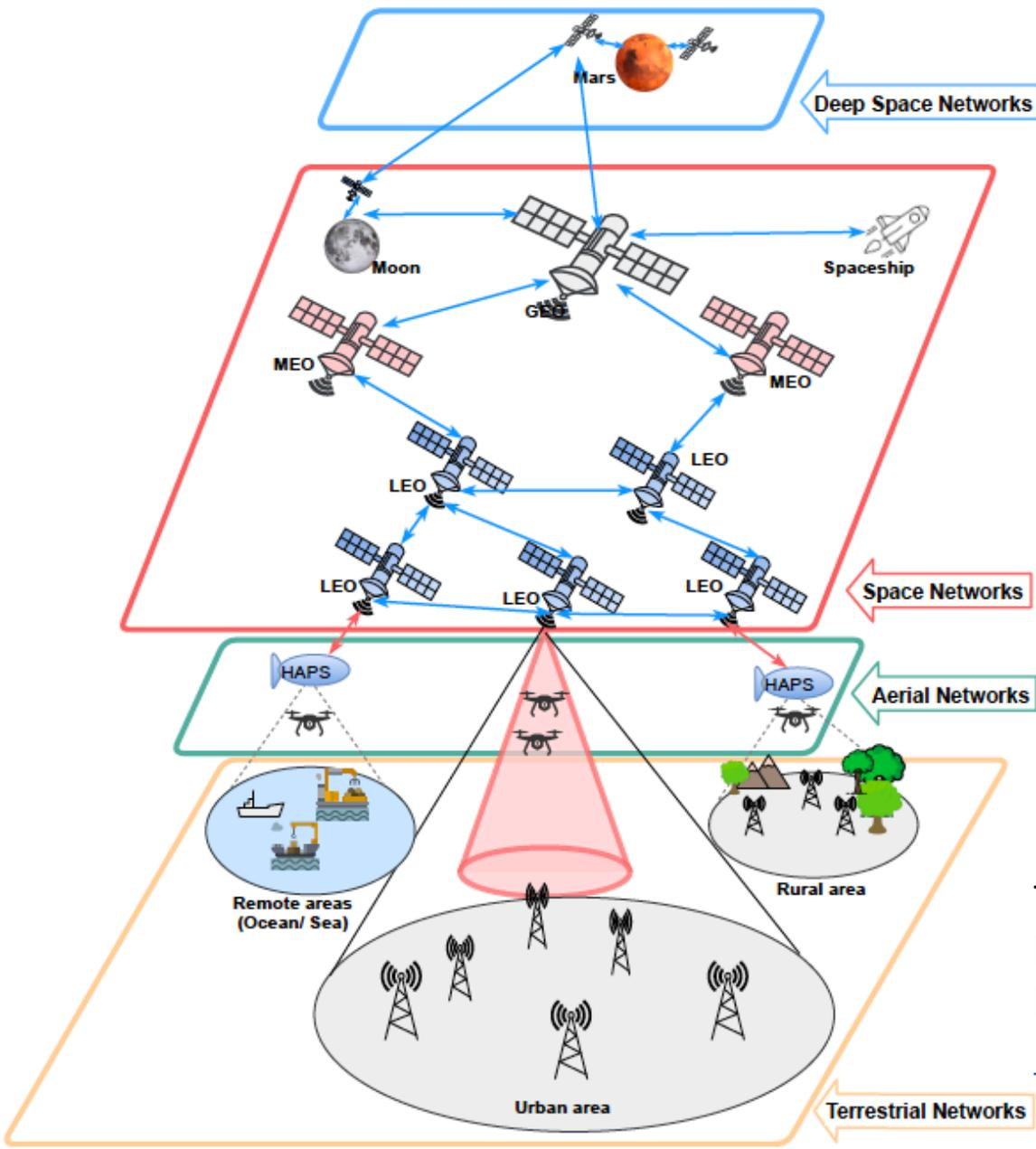
HAPS clusters serving as **Satellite Network Interface** will fuel the integration of terrestrial and satellite networks
