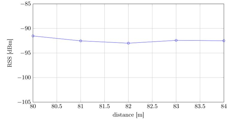
(b) Received Signal Strength at 434MHz
