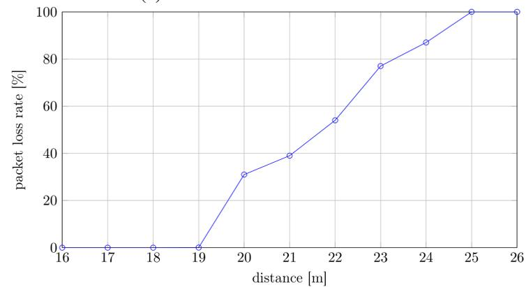
(c) Packet loss rate at 868MHz
