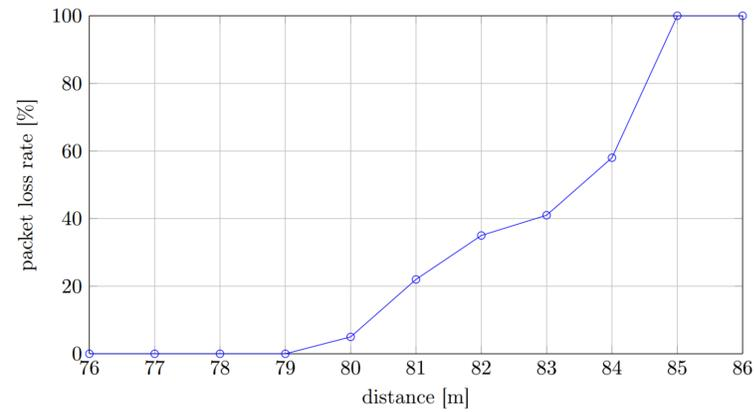
(a) Packet loss rate at 434MHz
