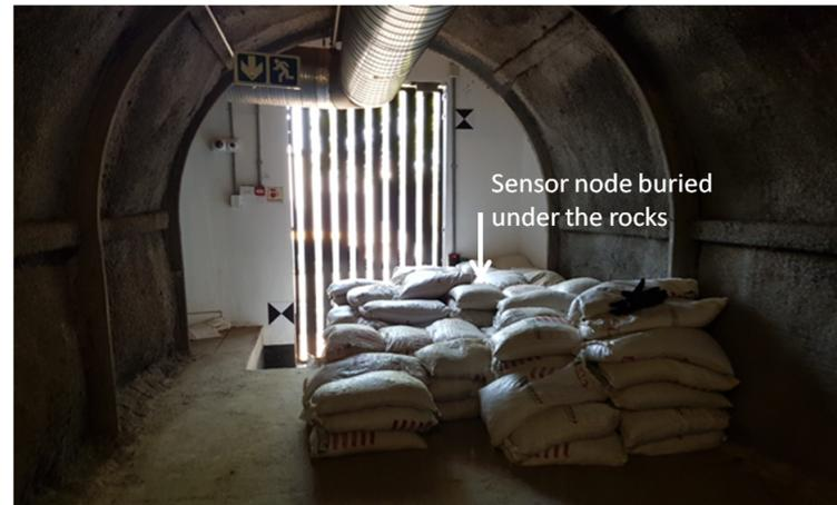
a) Sensor node buried under the emulated rockfall
