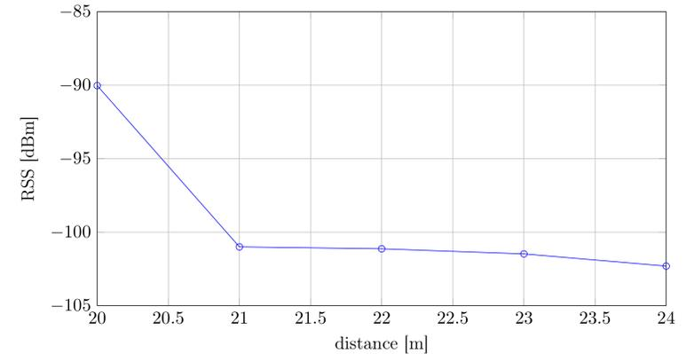
(d) Received Signal Strength at 868MHz
