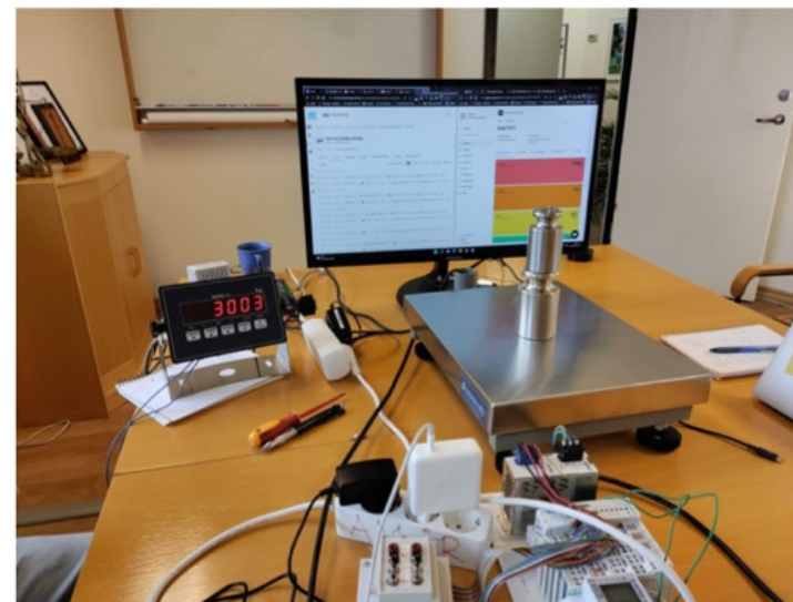
Fig. 2. An RS-485 enabled scale sending data using LoRaWAN to The Things Network and Datacake.
