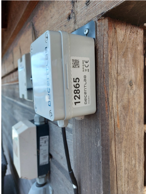
(a) Conductivity sensor (DL-CTD10)
