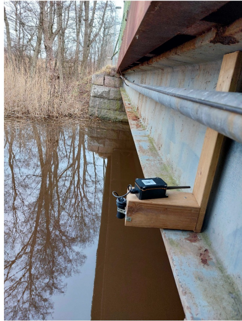
(b) Distance sensor (LDDS75)
