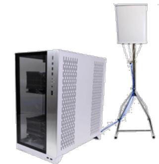
gNB (5G base station)
