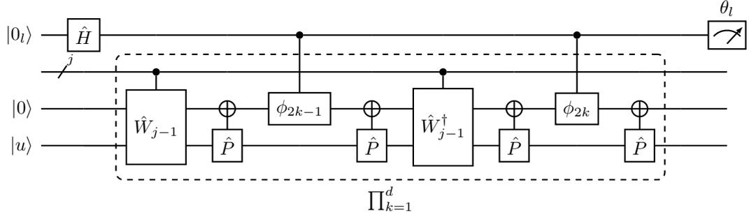
**Figure 2.** The  $l^{\text{th}}$  section of the QSVT quantum circuit for phase estimation algorithm, where  $\phi$  is a phase rotation gate which takes the rotation parameters as argument and the  $C_{\hat{p}}NOT$  and  $C_{\hat{p}'}NOT$  gates target the ancilla qubit. The expanded form of the  $\hat{W}_j$  can be found in<sup>7</sup>.
