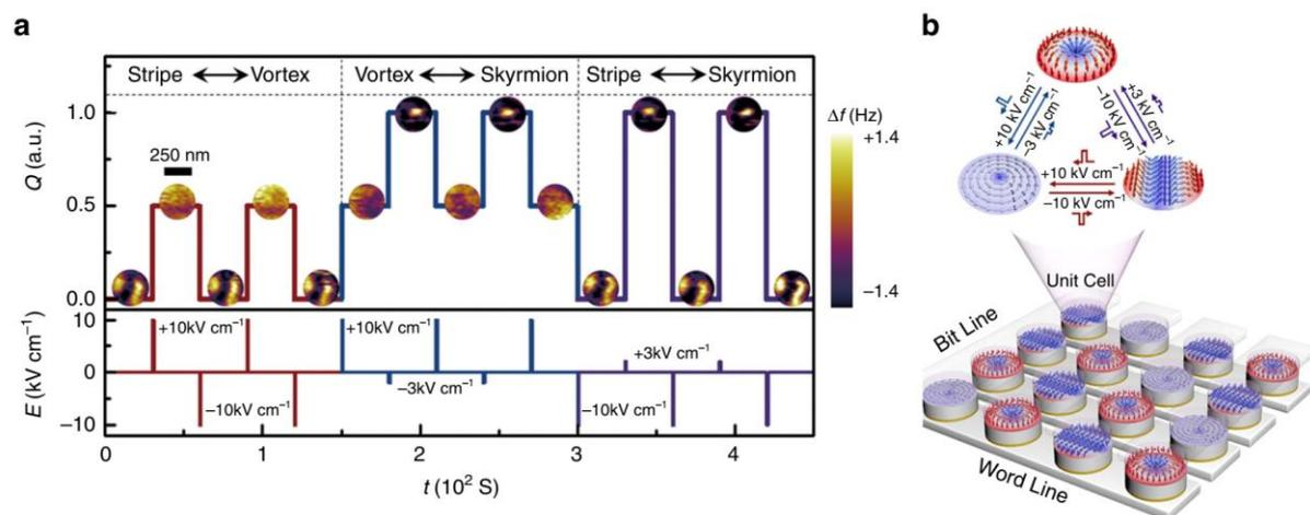
**Fig. 1.** Switching of individual skyrmions induced by pulse electric field.
