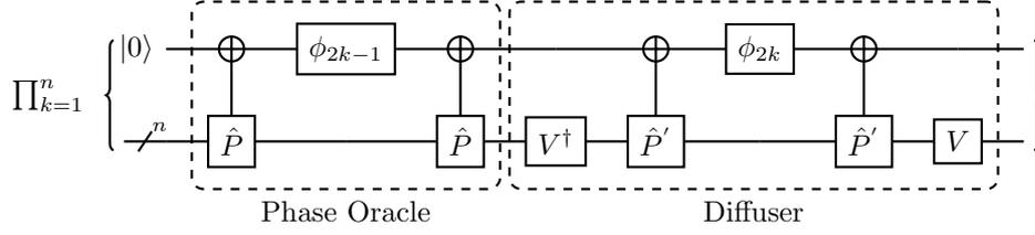
**Figure 1.** The QSVT quantum circuit for Grover search algorithm, composed of the phase rotation gate  $\phi$ , which takes rotation parameters as input, the unitary  $\hat{V} = \hat{H}^{\otimes n}$  operators and the  $C_{\hat{P}}NOT$  and  $C_{\hat{P}'}NOT$  gates that target the ancilla qubit.
