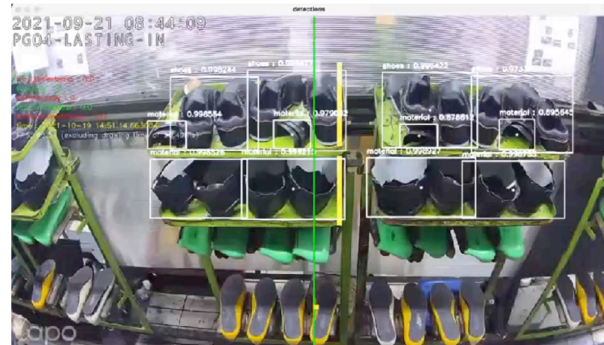
Exhibit #4: Parts and assembly line tracking : this can be used to monitor production output rate, reduce wait time, and energy consumption.
