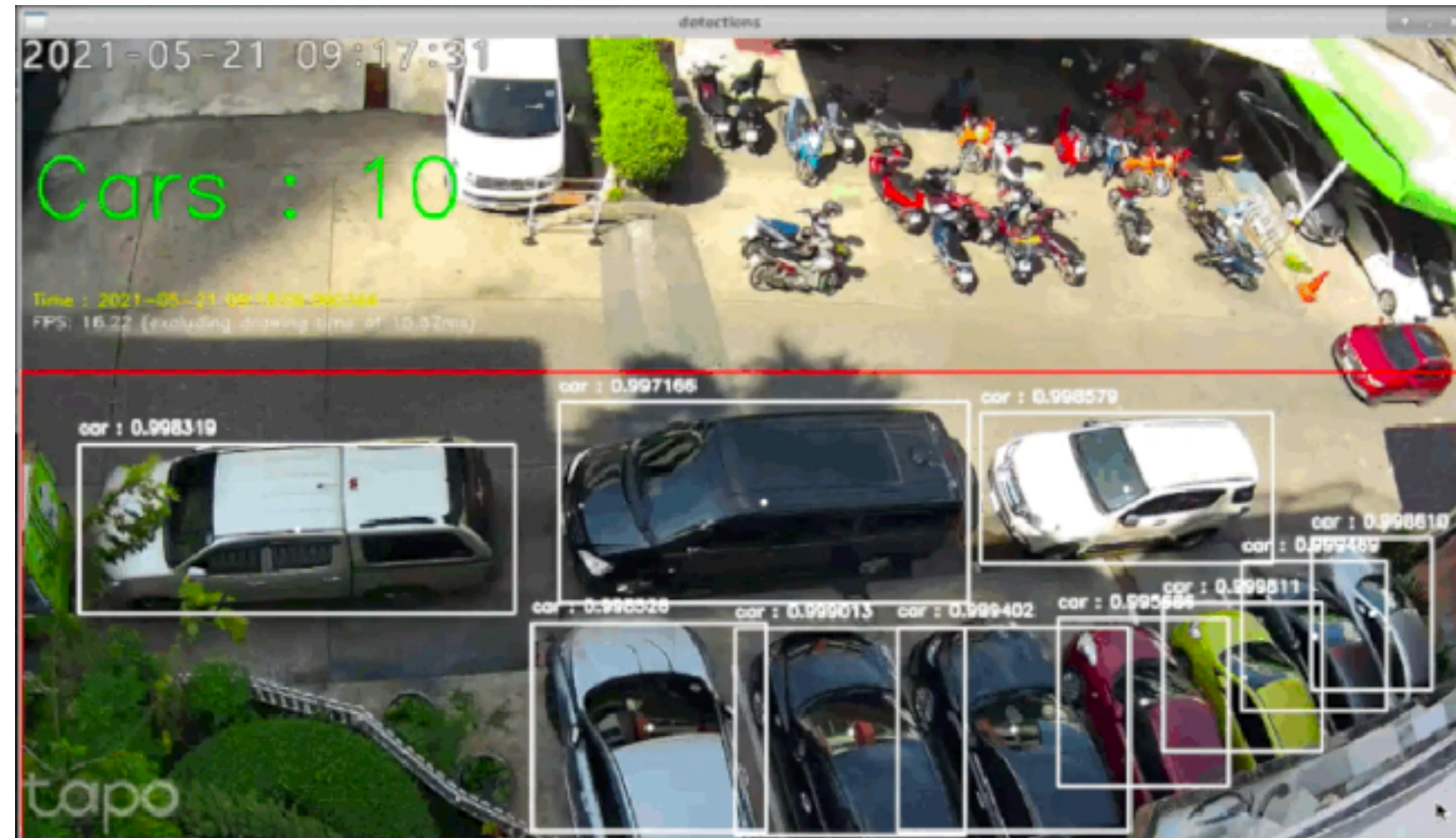
Exhibit #1: Vehicle space occupancy and parking wait time sensing: this can be used to schedule delivery or vehicle admission that aims to reduce fuel consumption.
