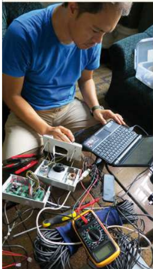
Reggie Mercado rigging a system of wires, cables, laptop and camera to look 20 meters down the hollow columns
