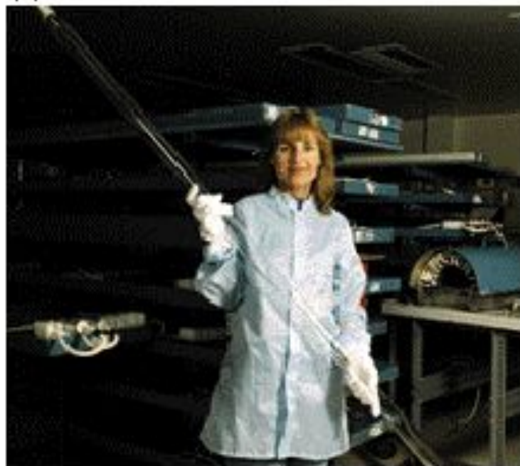
7680 flashlamps, each 6 feet long 30 kJ energy each
