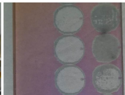
Damages left on plasma mirror by the interaction with the high-power laser beam.
