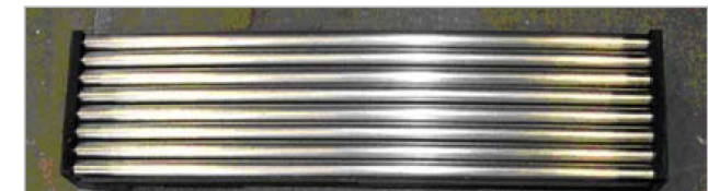
Figure 2.2 Tubes used in a proportional detector for large-area detectors. Source: Oak Ridge National Laboratory.
