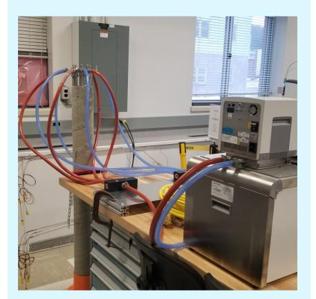
Investigate stresses induced by thermal gradients, a common driver for foundation and tank failure in two-tank nitrate molten salt storage systems.
