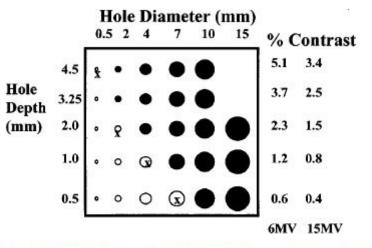
FIG. 10. Aluminum Las Vegas phantom for EPID image contrast and spatial resolution.
