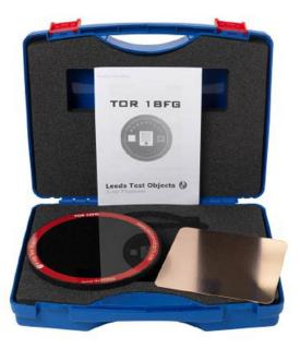
Phantom designed for fluoroscopy
