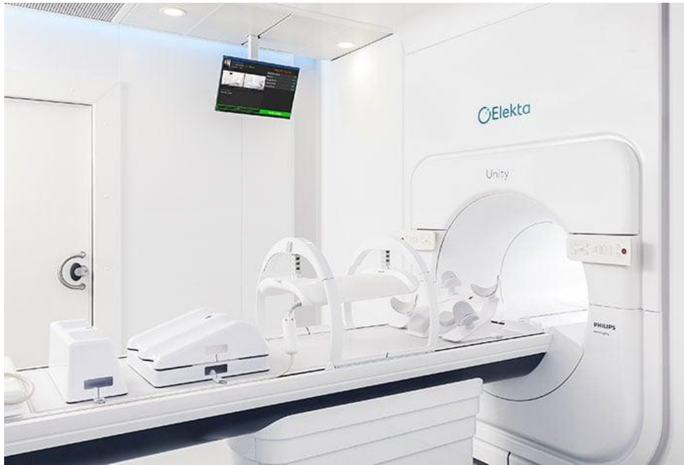
Elekta Unity: 7 MV FFF linear accelerator mounted in a ring around a 1.5 T closed superconducting magnet, SAD: 145 cm, field size of 55 x 29 cm
