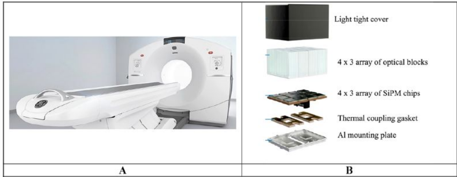
Fig. 1. (A) Picture of the GE Discovery MI PET/CT. (B) Picture of a 4x3 array of optical blocks coupled to a 4 × 3 array of SiPM chips [52]. Each optical block is a 4 × 3 array of 3.95 \times 5.3 \times 25 \text{ mm}^3 Lu-based pixels and each SiPM chip is 3 × 2 pixel array with pixel size of 4 \times 6 \text{ mm}^2 .
