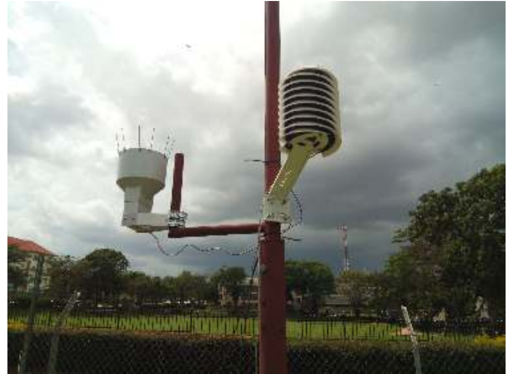
LoRaWAN Meteo station with rain gage in Kampala, Uganda
