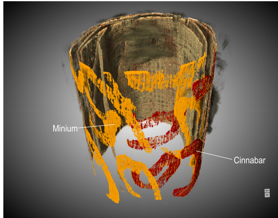
Absorption edge sensitive tomography \text{Pb}_3\text{O}_4 and \text{HgS}
