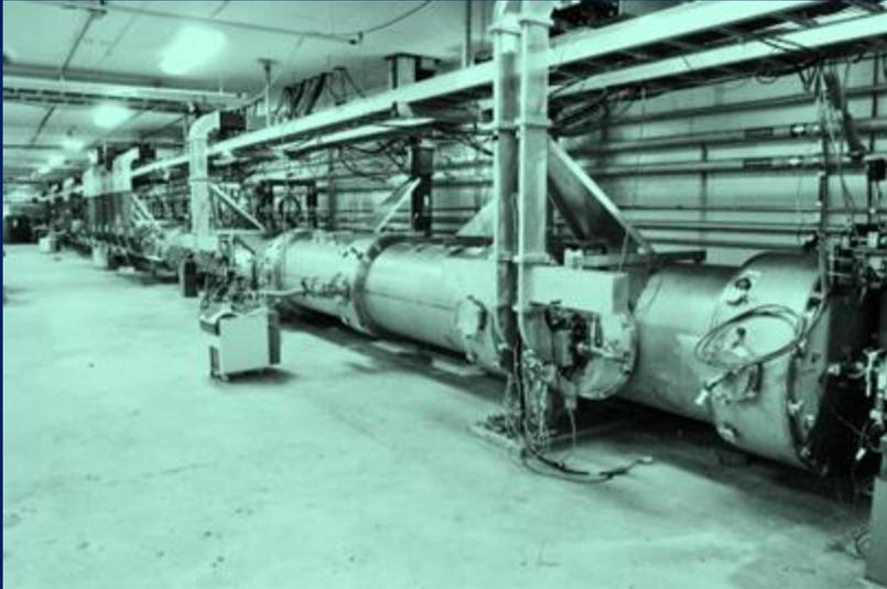
...to emit x-rays, high-energy electrons with large  $\gamma$ -values are required, whose relativistic “longitudinal mass”  $\gamma^3 m_0$  is very heavy: it takes a (relatively) long time to shift them to the “slices”, so **a very long undulator is required for microbunching**
