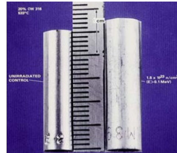
Figure 6-24. Easily observed swelling ( \approx 10\% linear, \approx 33\% volumetric) in unfueled 20% cold worked AISI 316 cladding tube at 1.5 \times 10^{23} \text{ n cm}^{-2} ( E > 0.1 \text{ MeV} ) or \approx 75 \text{ dpa} at 510^\circ \text{C} in EBR-II (after Straalsund et al., 1982). Note that, in the absence of physical restraints, all relative proportions are preserved during swelling.
