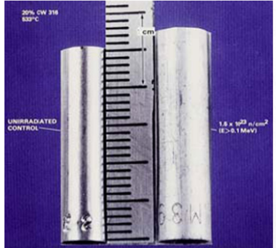
Figure 6-24. Easily observed swelling ( \approx 10\% linear, \approx 33\% volumetric) in unfueled 20% cold worked AISI 316 cladding tube at 1.5 \times 10^{23} \text{ n cm}^{-2} ( E > 0.1 \text{ MeV} ) or \approx 75 \text{ dpa} at 510^\circ\text{C} in EBR-II (after Straalsund et al., 1982). Note that, in the absence of physical restraints, all relative proportions are preserved during swelling.
