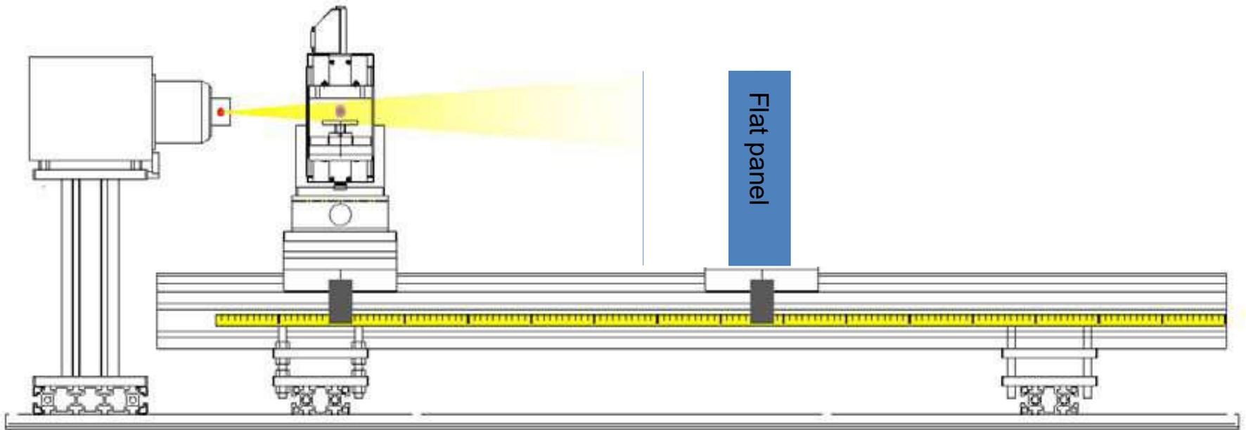
The source-detector system and the sample manipulator are mounted on a flexible mechanical set-up
