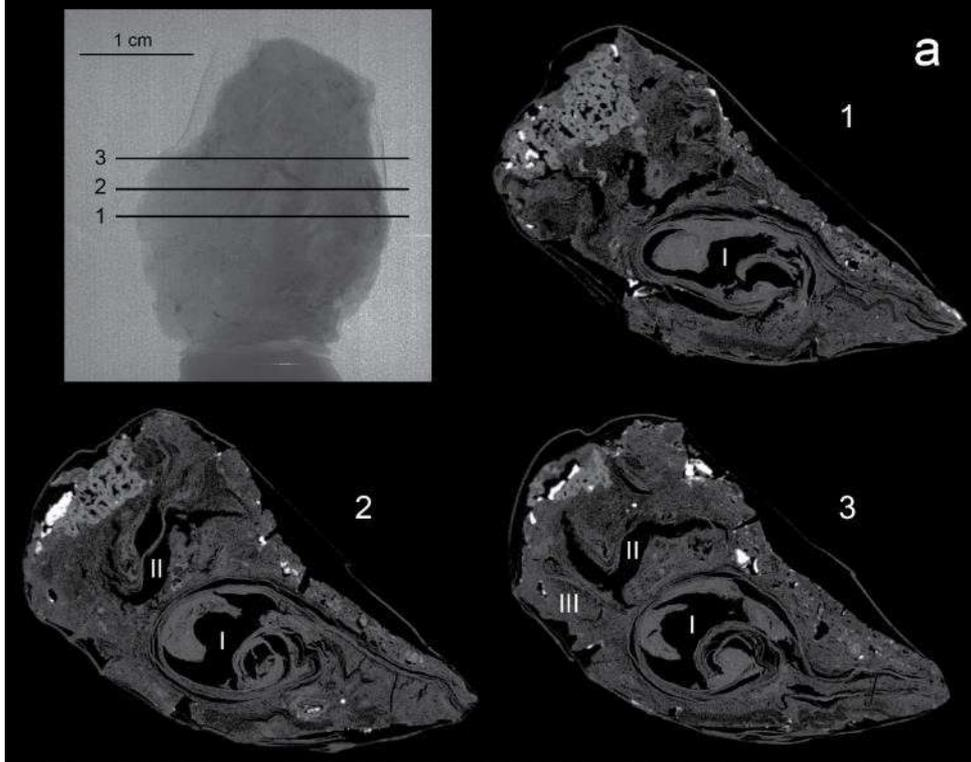
(a) MicroCT virtual sections of sample CORT, showing its scroll-up structure. (b) Birch bark rolls. The birch bark naturally curls into loose rolls when it is removed.
