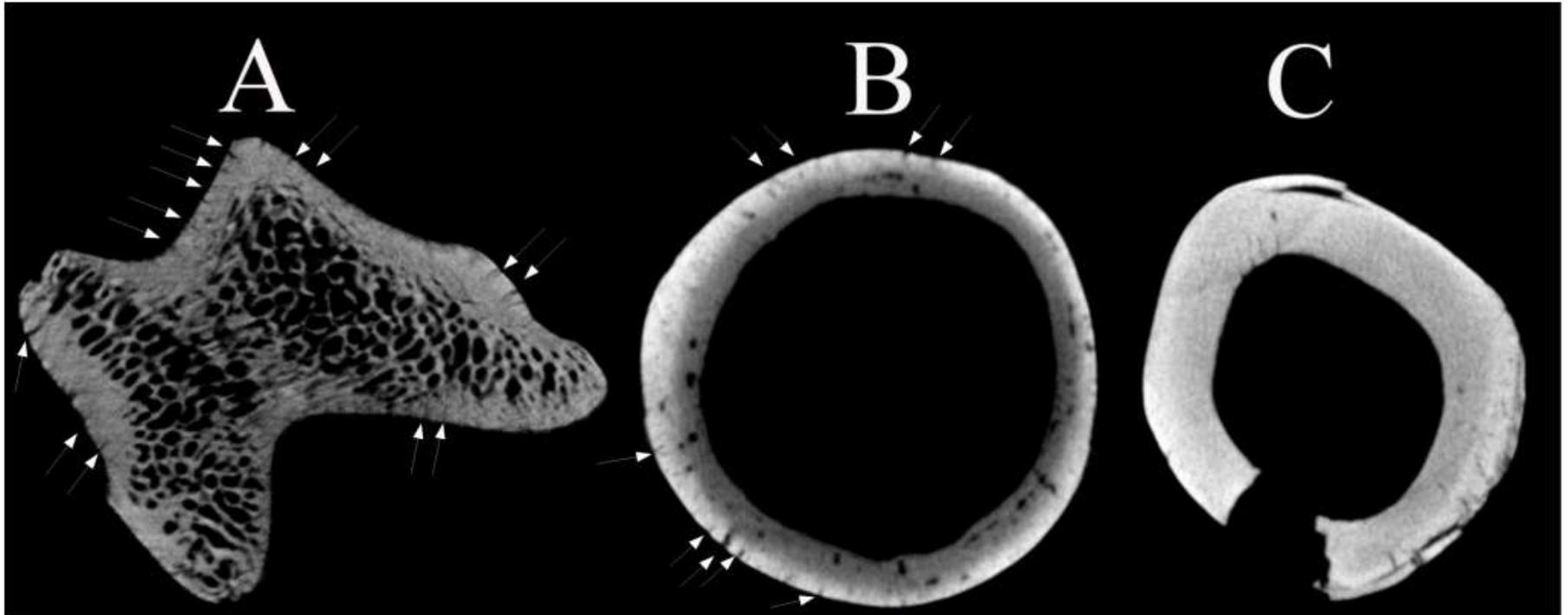
**Figure 3.** Cross-sections of burned specimens 1 (A), burned at 600°C, 4 (B), burned at 900°C, and 5 (C), burned at 900°C. Thin cracks perpendicular to the outer surface are visible in the cortical region of specimens A and B (white arrows). Cracks parallel to the outer surface, related to bone deformation, are visible in C. A change in greyscale values from the marrow cavity to the outer surface (indicating an increase in bone density) is visible in B.
