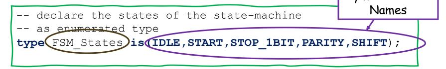
Declare the signals for the next state and current state of the state machine as signal of the enumerated data type already defined for the state machine
