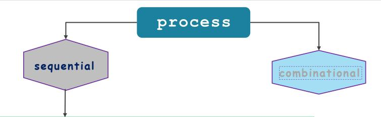
A clock-controlled process, also known as a **sequential process**, describes logic whose outputs change only at specific edges of a clock signal (e.g., rising edge or falling edge). This type of process is used to model sequential elements like flip-flops, registers, counters, and state machines, which have memory and store state.
