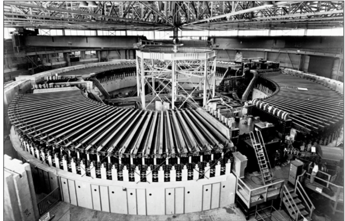
The 6 GeV proton synchrotron (Bevatron) at UC Berkeley in 1954
