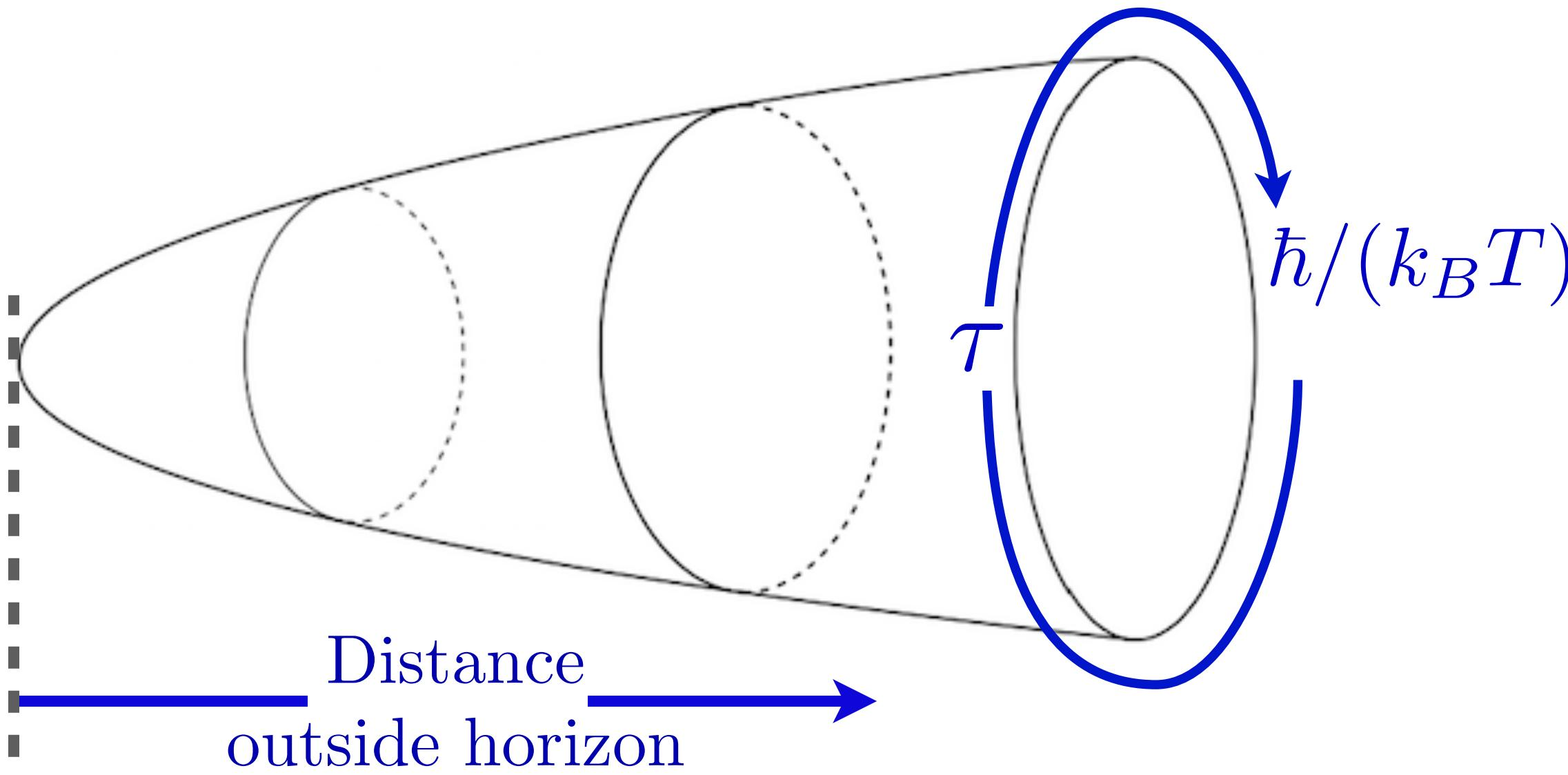
The  $T > 0$  quantum partition function is obtained in a spacetime which is periodic as a function of  $\tau$  with period  $\hbar/(k_B T)$ . We have to ensure that there is no singularity at the horizon  $r_0$  where  $V(r_0) = 0$ . Let us change radial co-ordinates to  $y$ , where  $r = r_0 + y^2$ . Then for small  $y$
