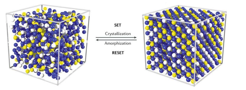
Large difference in properties between the two phases
